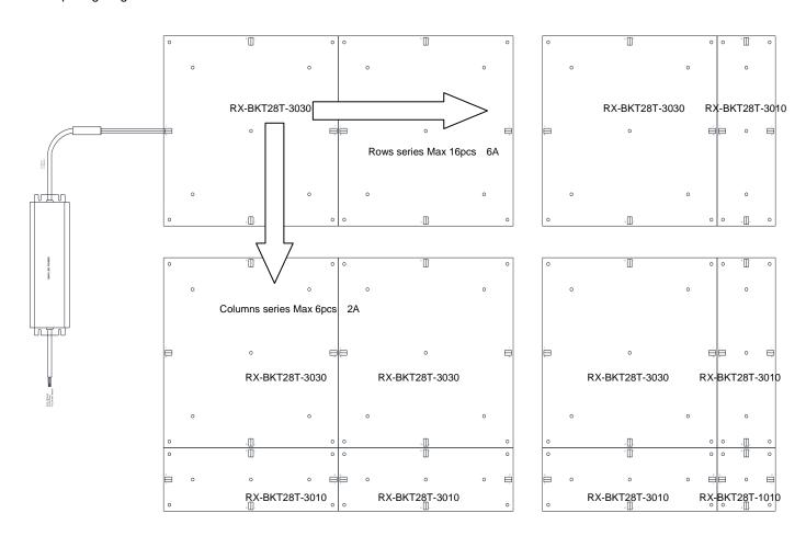
Note: Row and column totals; must be less than the number of LED module can be spliced (RX-BKT28T-3030: Row QTY x Column QTY ≤16pcs)
