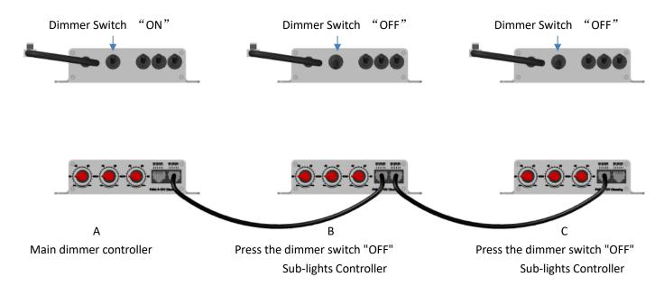
Step I, Conect multiple lights with RJI I/12 cable(suport up to 12 lights)
