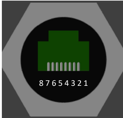
CH1 Dimming signal input : Pin 1 DIM+, Pin 2 DIM-
