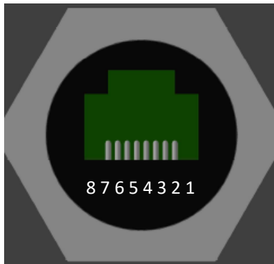
RJ45 socket Dimming connector
